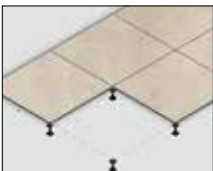
Installation as a raised paving
